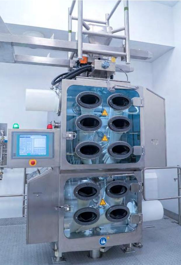
Roller compaction turns powder blends into densified sheets using the pressure of two compacting rollers. The resulting sheets can then be milled to any desired mesh size providing an efficient and scalable process. PCI has invested in contained Gerteis Mini-Pactor technology to further expand our contained manufacturing operations. This technology offers a patented proven design able to process highly potent molecules using effective containment technology and integrated cleaning systems.
